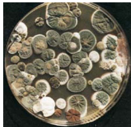
Compressed air sample from oil lubricated compressor without drying of the air. After cultivation a large concentration of various germs was discovered.
