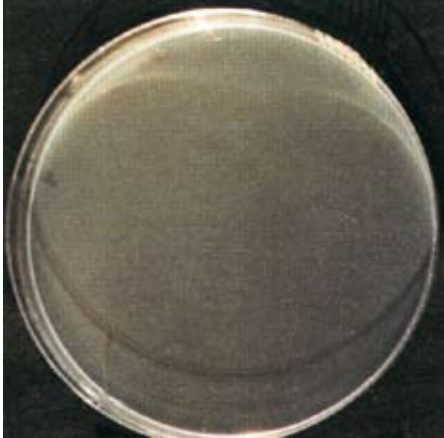
Compressed air sample from oil less compressor with adsorption air dryer. After cultivation no bacteria was to be found.
